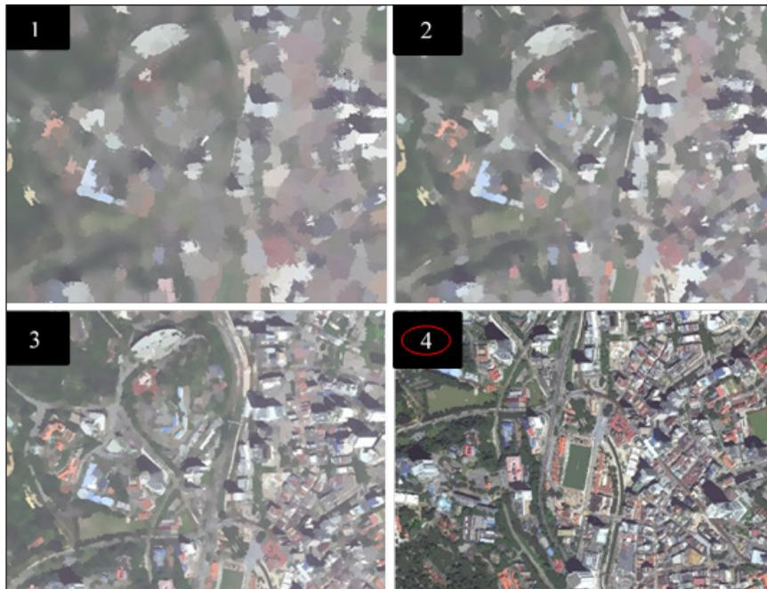
Figure 4. Image segmentation processing with different parameter testings through segment-mean function algorithm. Test 4 image indicated significant results.
